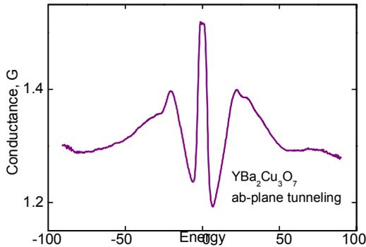
**FIGURE 9.** Tunneling conductance of a high- $T_c$  superconductor. Note how different this appears from the BCS conductance in the previous figure. The zero-bias conductance peak arises from Andreev bound states, due to the broken reflection symmetry of the superconducting order parameter, as discussed in the text. After Greene et al., 2000.
