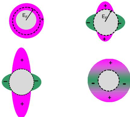
**FIGURE 14.** Pure (*top*) and mixed (*bottom*) order parameter symmetries. The first mixed state is d+s, which is energetically un-favorable. The second is d+is, which is favored. Note the continuous change of the order parameter on the Fermi surface of the d+is state, which indicates that this state spontaneously breaks time-reversal symmetry. After Greene et al., 2000.
