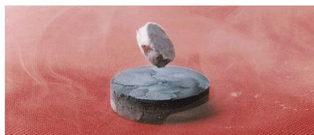
**FIGURE 3.** Magnetic levitation by a high-temperature superconductor. From <http://research.cm.utexas.edu/jmcdevitt/>.
