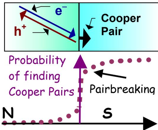
**FIGURE 10.** Andreev reflection. *Top:* An electron incident on a superconductor is retro-reflected as a hole, as described in the text. *Bottom:* this AR process is the microscopic explanation for the superconducting proximity effect. Some phase coherence is generated on the N side with pair breaking on the S side. The length scales are proportional to the electron coherence length in each material. This is the ONLY example of a clean SN interface in this talk.
