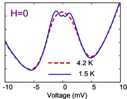
**FIGURE 13.** Spontaneous splitting of the zero-bias conductance peak observed as a signature of spontaneous time-reversal symmetry breaking in a superconductor. After Greene et al., 2000.
