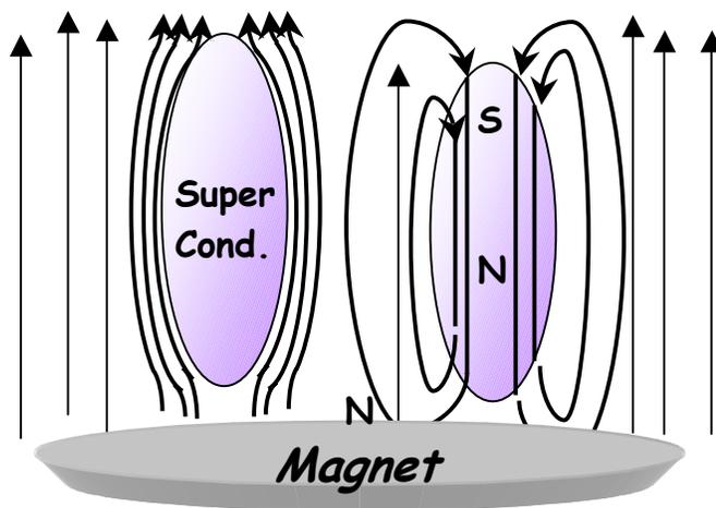
**FIGURE 2.** Meissner-Ochsenfeld Effect. Magnetic field lines are expelled from the superconductor due to supercurrents forming on its surface. This diamagnetism leads to magnetic levitation.
