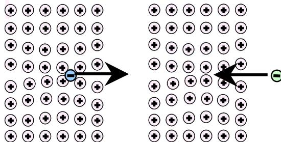
**FIGURE 1.** Schematic of the electron-phonon momentum-space pairing basis for Cooper pairs. The first electron, traveling to the right, leaves a "positive wake" in the lattice which, with a time delay, attracts the second electron. After Simon and Smith, 1988.
