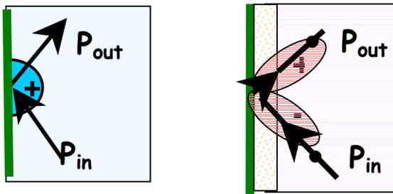
**FIGURE 12.** Surface reflection within a superconductor. For an  $s$ -wave superconductor (*left*), no change of the OP is seen so no AR occurs. For a  $d$ -wave superconductor (*right*) for certain surfaces, the electron experiences a sign change of the OP upon reflection so a dramatic AR occurs resulting in pair breaking near the interface.
