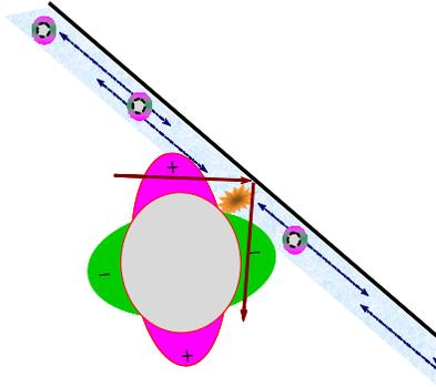
**FIGURE 15.** Representation of the broken time-reversal symmetry state at the surface of a d-wave superconductor. Note the d+is OP near the surface and the subsequent flow of electrons, represented by vectors along the interface in the near-surface region.
