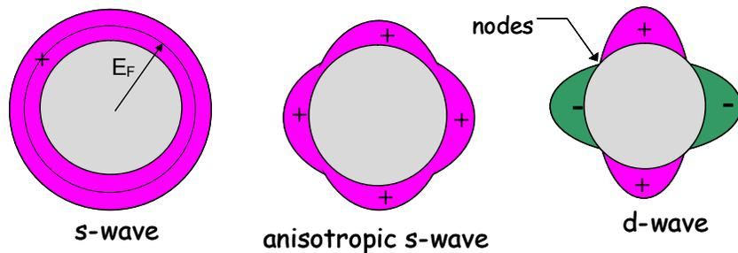
**FIGURE 11.** Three possible order parameter symmetries: left to right  $s$ -wave, extended or anisotropic  $s$ -wave, and  $d$ -wave are shown. The first two are considered “conventional,” and most metallic superconductors exhibit  $s$ -wave order parameter symmetry. The high-temperature superconductors exhibit  $d$ -wave symmetry and are called unconventional because there is a sign change of the OP around the Fermi surface.
