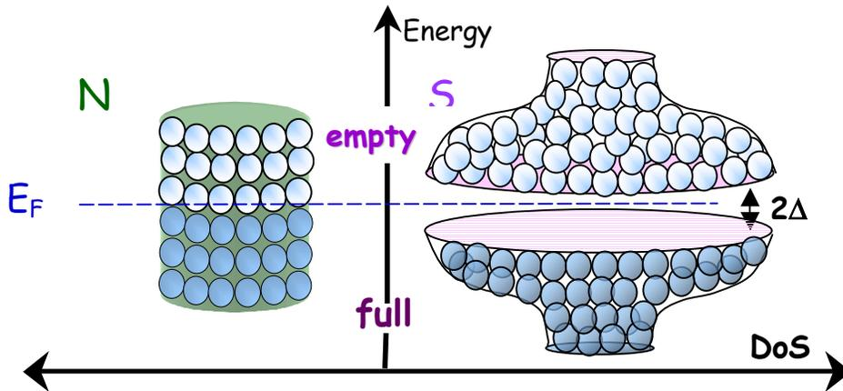
**FIGURE 7.** Schematic of the density of electronic states for a normal metal (N) and a superconductor (S). At low temperature the electrons fill to the Fermi level, and the energy gap in the superconductor,  $\Delta$ , is nominally the binding energy of the Cooper pairs. After Simon and Smith, 1988.
